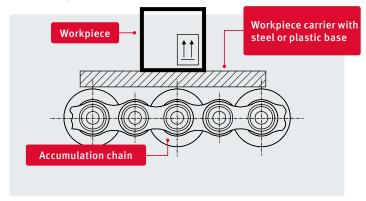
Losses due to friction occur at the following chain drive components: Chain, chain tensioner, chain guide, sprocket, workpiece carrier and transported goods.
