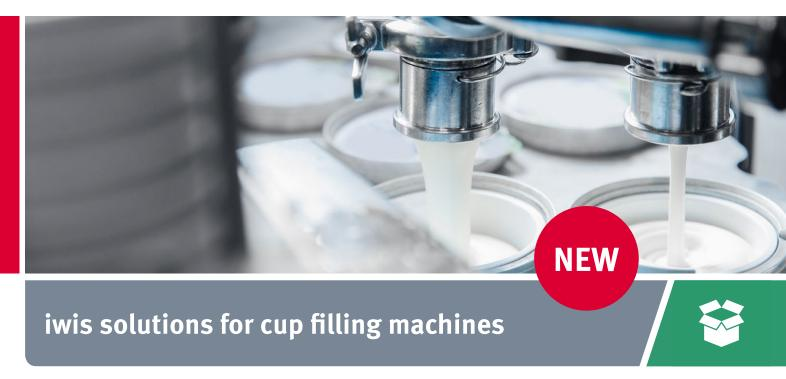
In the **food industry**, flexible and highly efficient pots filling machines are used to automatically and precisely fill milk and milk-based products such as yoghurt into pots. Cup filling machines use **stainless steel chains with cell plate adjusters** to convey the cup filling containers in order to position pots and trays under the dosing mechanism with pinpoint accuracy.
