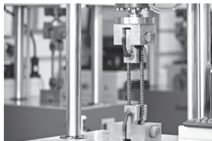
More than 15 pulser are available for testing dynamic fatigue strength according to different testing methods
