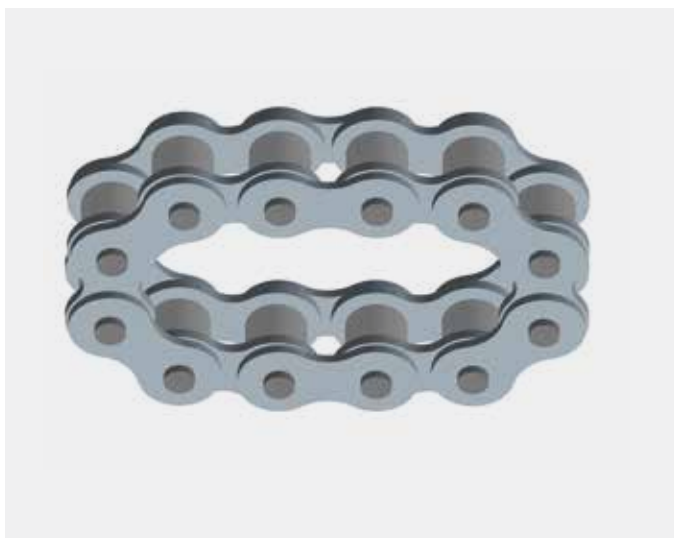
环形铆接滚子链需使用偶数链节 Continuously riveted endless roller chains require an even number of links
