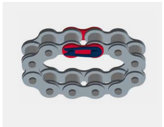
环形带接头滚子链需使用偶数链节（包括一个标准接头） Continuously endless roller chains require an even number of links, including a straight connecting link
