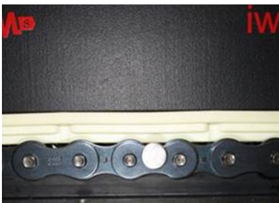
Magnet is mounted flush with the upper edge of the outer link plate.
